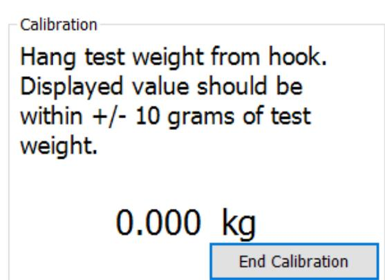
7. Check displayed value is within +/- 10 grams of test weight. Click **End Calibration** to continue using the penetrometer.
